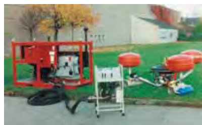
'Power packs' that can easily be moved to particularly vulnerable sites. The power packs are ready with engine, skimmer, pump and booms.
