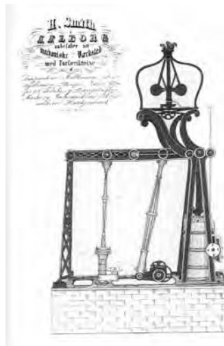
Steam machine for pump systems at the liquor factories 1844
