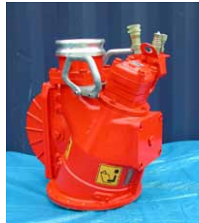
This pump is a vertical Archimedes screw pump that 'screws' the thick oil through the pump. When the operation takes place in arctic waters the oil is mixed with ice.
