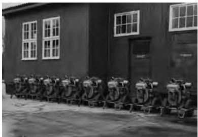
Small self-priming horizontal centrifugal pumps for readiness and defense purposes, 1947.
