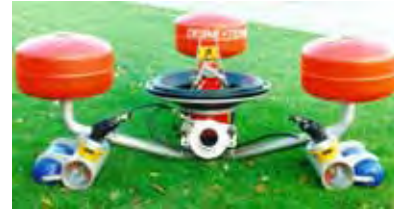
The picture shows a skimmer before use. The red pontoons enable the pump in the middle to float.
