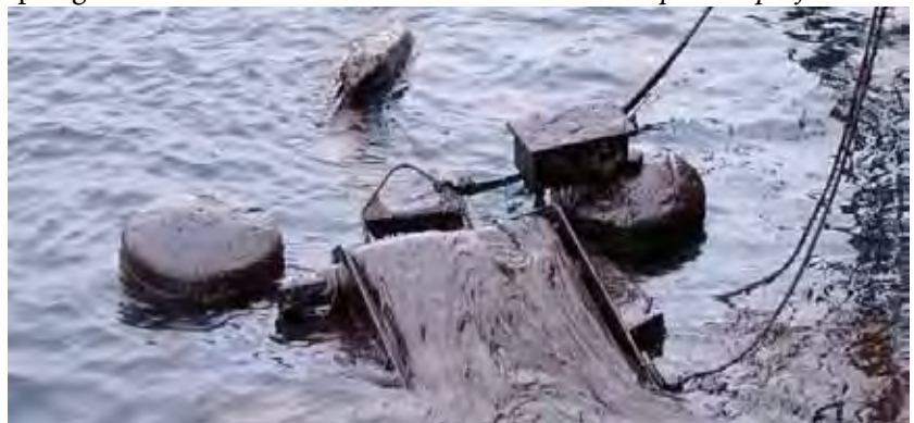
When the oil floating on the sea is contained it is removed by a 'skimmer' such as the one in this picture.
